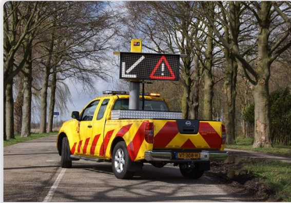
VEHICLE-MOUNTED TRAFFIC SIGNS
