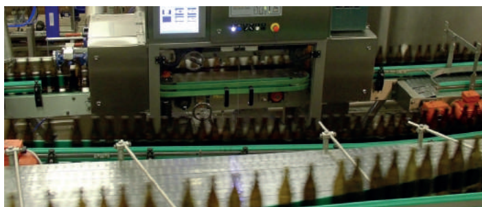
Filling line with UniscanBOTTLE installed
