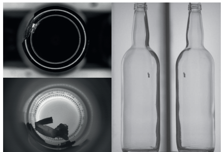
Detected defects on a bottle neck (left) and inside a bottle (right)
